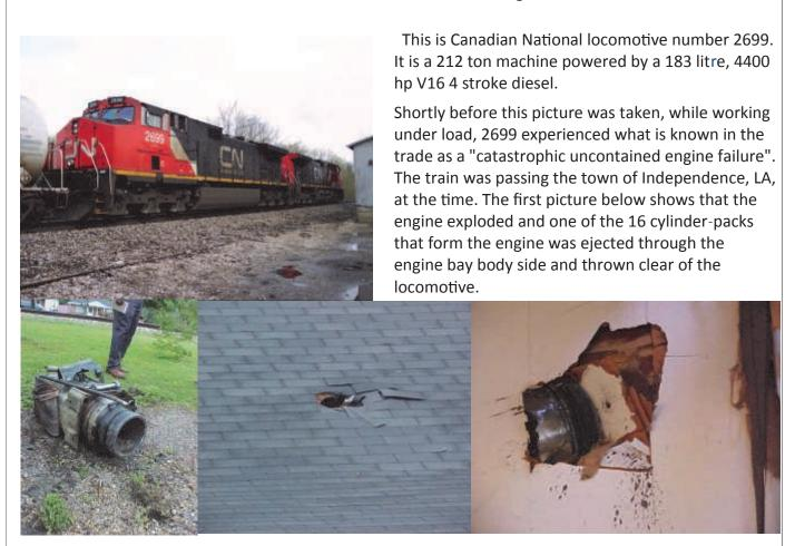
In addition to this the piston from that cylinder was thrown free by the force of the failure. It was ejected so violently that it travelled through the air and crashed through the roof of a nearby home where it imbedded itself in an interior wall.
